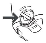
To regulate the ionization power even more precisely, you can also change the flow rate of the water. For this purpose, a ceramic valve is attached to the underside of the **ECAIA container S** (2-B) attachment container, which can be opened and closed. The more you close the ceramic valve, the slower the flow rate. Keep in mind: The slower the flow, the stronger the ionization.
