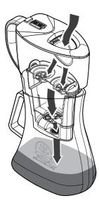
Then place the additional **ECAIA container S** (2-B) on the **ECAIA glass jug S** (2-A). As an alternative to the glass carafe, the tank container **ECAIA tank S** (2-C) can also be used. Note that the capacity of the tank is only 0.45 liters. Wait until all the water in the additional container has flowed through the filters into the glass carafe or tank container.
