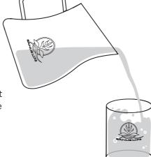
**Note**: To ensure optimal filter performance, it is recommended that the **ECAIA main filter S** (2-E) cartridge be completely submerged in water and shaken vigorously once a week, or as soon as the water flow decreases significantly. This prevents the activated carbon from clumping and optimizes the water flow.
